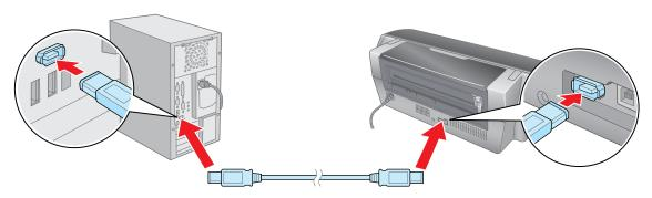
NOTE: If your computer uses i.Link or another 4-pin FireWire connection, you will need to connect a 6-pin to 4-pin FireWire (IEEE 1394) cable.
